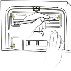
MARK THE POSITION TO DRILL WALL MOUNTING HOLES.
