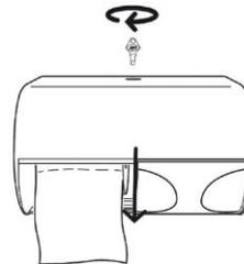
CHIUDERE IL DISTRIBUTORE E ASSICURARSI CHE IL MECCANISMO DI BLOCCAGGIO SI INNESCHI.
